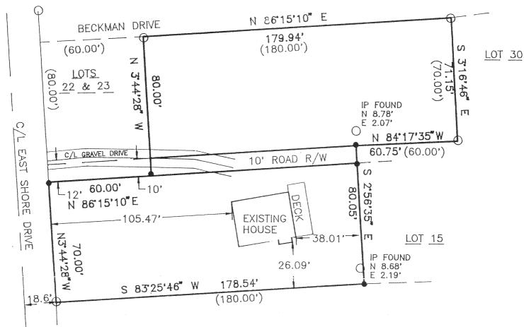
The above map is a true representation thereof and shows the size of location of all the property, exterior boundaries, the location of all visible boundary fences, apparent easements, roadways and visible encroachments, if any.
